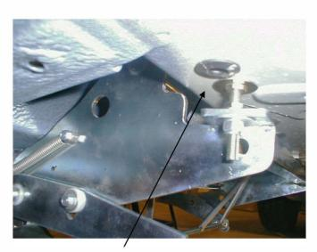
MAYBE NECESSARY TO DRILL 010 FIXING HOLE IN THE CHASSIS AL THOUGH PREFERRED METHOD JS TO USE EXISTING CHASSIS HOLE
