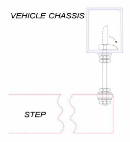
LOCATE CHASSIS HOLES USING THE TOGGLE FIXINGS SECURE THE REAR OF THE STEP BY PLACING THE TOGGLE THROUGH THE CHASSIS HOLE AND ALLOWING TOGGLE TO BRACE THE HOLE
