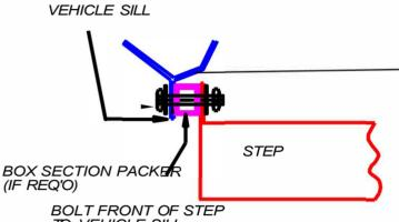
TO VEHICLE SILL USING BOX SECTION PACKER(IF REQ'D) MB BOLTS/NUTS &WASHERS
