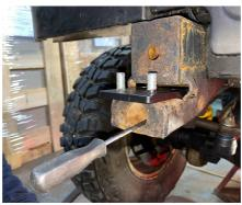
**6.** The lower section of the extension bracket can be fitted into the Chassis Bumper connection
