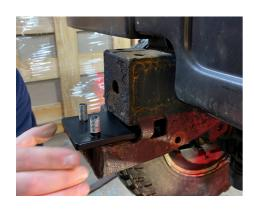
**5.** Now Insert the lower half of the extension bracket into the Chassis **bumper Connection**
