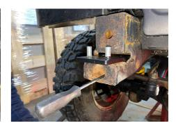
**4.** Carefully position the nut insert
