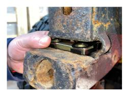
**2.** Before fitting the bottom piece of the extension bracket into the chassis, the nut insert needs to be carefully placed in
