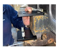
**7.** Position the top section of the extension bracket and insert 2 bolts through the screw holes to secure the extension bracket to the chassis.
