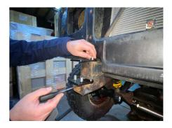
**10.** Tighten the bolts to secure both parts of extension bracket to the chassis.
