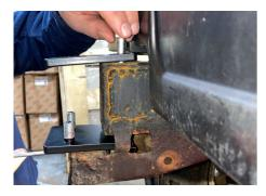
**8.** Carefully manoeuvre the nut insert until the securing bolts can be secured into it.
